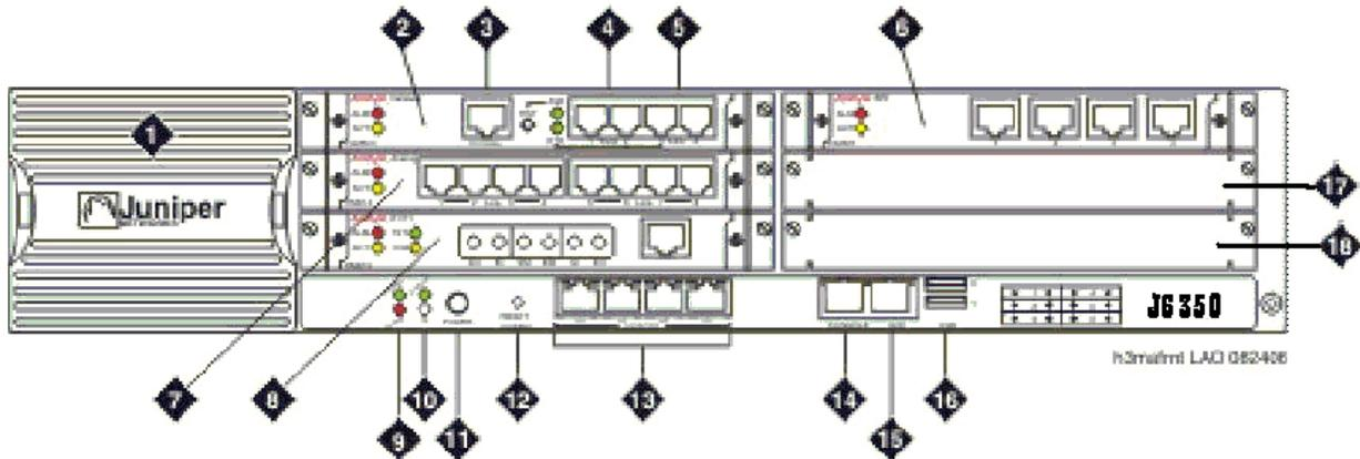
Figure 3: IG550 Integrated Gateway in a J6350 Services Router
