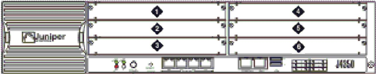
The J4350 Services router chassis has six slots. Modules can be inserted into the slots according to the following guidelines:
