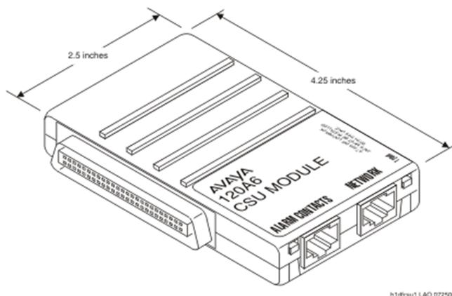
**Figure 6:** This figure shows the 120A channel service unit.
