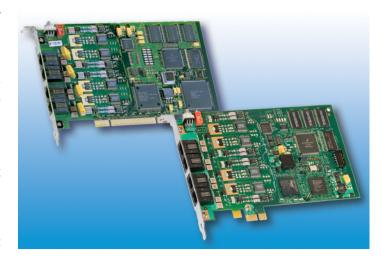
a telephone trunk line; Caller ID is supported for North America (CLASS protocol), the United Kingdom (CLI protocol), and in Japan (CLIP protocol). Features such as fax and software-based speech recognition processing enable unified messaging applications. They also provide Automatic Gain Control (AGC), so even a weak telephone signal can be recorded and replayed with clarity.
