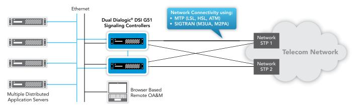
Figure 1. Dialogic® DSI G51 Signaling Controllers in a Service Provider Network
